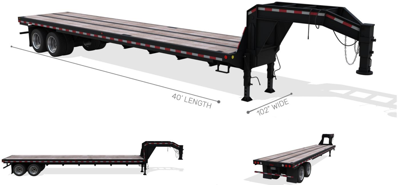
Hot Shot Trailers are primarily used to transport shipments that are lower in overall weight, usually up to approximately 15,000 lbs, but that also need to travel on an open trailer in order to be side loaded, rear loaded or loaded from above. These trailers are typically pulled using a Pick Up Truck or a similar type vehicle. Deck lengths vary and are most often between 30' and 40' in length. The low profile of the deck allows for freight height of between 120" and 130" in most cases.
