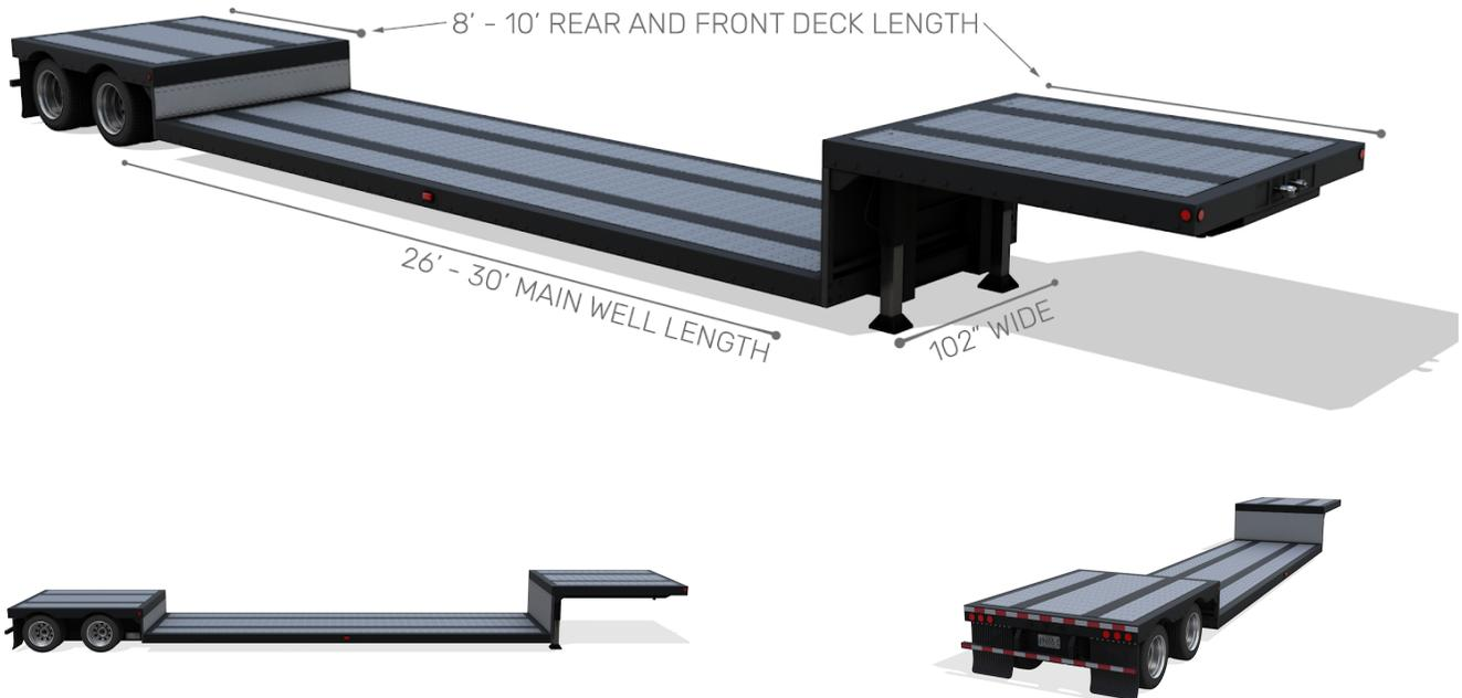
Double Drop trailers, also known as Low Boys, are utilized to transport oversized freight both legally, and through the use of permits and/or escorts. There are three decks: the upper deck, the lower deck and the well. The well allows for freight up to 144" high to be legally transported. There are a number of trailer variations which allow for the transport of a wide array of oversized freight with varying degrees of length and height. Full tarping options are available as needed.
