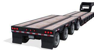
A Removable Gooseneck Trailer (RGN) is utilized to transport larger shipments both legally, and through the use of permits and/or escorts. They are primarily used to transport equipment that needs to be driven on or off of the trailer. Units such as farm equipment and specialty vehicles are commonly shipped on RGNs. The removable gooseneck can be separated from the cab allowing access to the drop down ramps of the trailer to allow for the units to easily be driven on or off.
