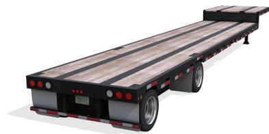
Step Deck trailers are primarily used to transport products that are too tall for a normal Flatbed trailer. There is an upper deck and a lower deck. The lower deck, called the well, allows for freight up to 120" high to be legally transported, while still providing the same loading/unloading capabilities of a standard Flatbed trailer. Specialized Low Pro Step Decks can manage freight that is up to approximately 126" to 128" in height.
