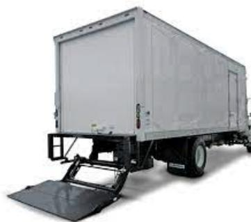
Similar to Dry Vans as they allow for dock-level loading/unloading and protect product from the elements. The main difference is in the capacity. A Straight Truck is typically 20' to 28' in length which is ideal for picking up or delivering to locations where space is limited. Many Straight Trucks are equipped with Tailgates that allow for ground-level access where no dock is available.
